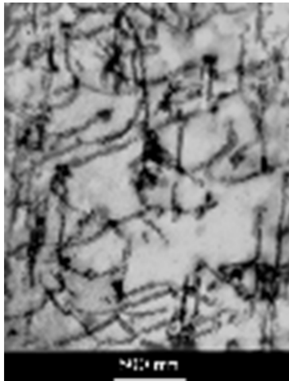
Figure 11: Tempered martensitic steel structure with precipitation of Mo -Fe, C 0.2, Mo 4.
