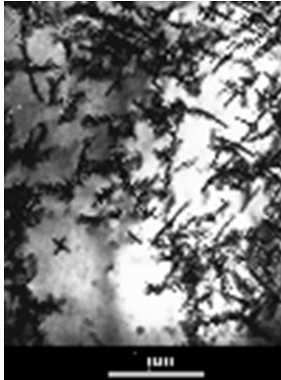
Figure 8: Tempered martensitic steel structure with precipitation of Mo -Fe, C 0.2, Mo 4
