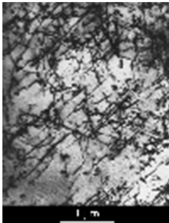
Figure 9: Tempered martensitic steel structure with precipitation of Mo -Fe, C 0.2, Mo 4.
