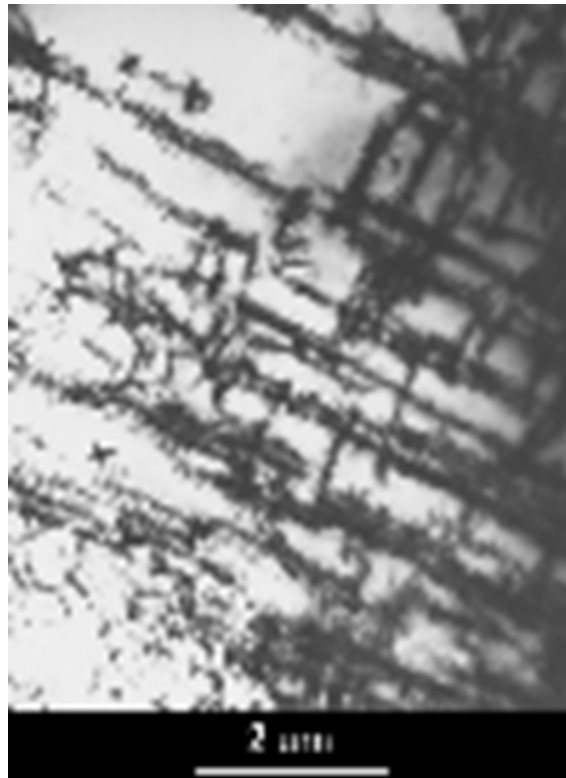
Figure 12: Tempered martensitic steel structure with precipitation of Mo -Fe, C 0.2, Mo 4.
